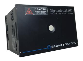
For the ultimate in resolution and accuracy, the SpectralLED® 940-SWIR source incorporates 16 discrete LED devices, all with a center wavelength of 940 nm. The output is directly coupled into a 38mm diameter homogenizing rod, with a length of 190 mm, having a diffuser optically bonded to the output surface.
