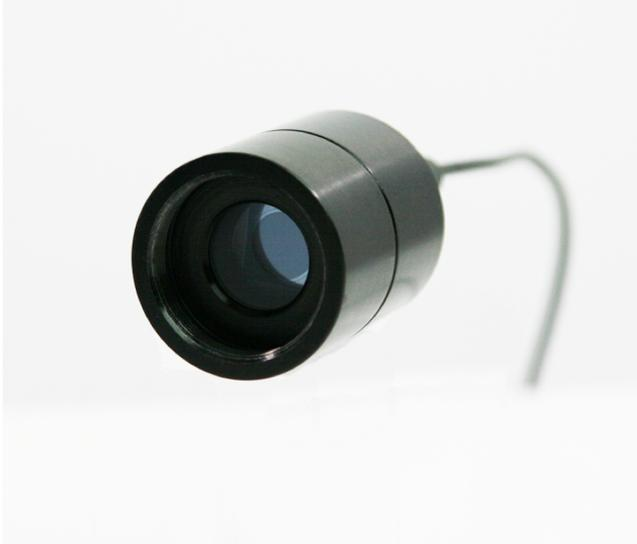
The model 247 radiometric sensor includes a precision radiometric filter for flat response from the blue to the near-infrared. This sensor assembly is popular for its high linearity and low noise performance.
