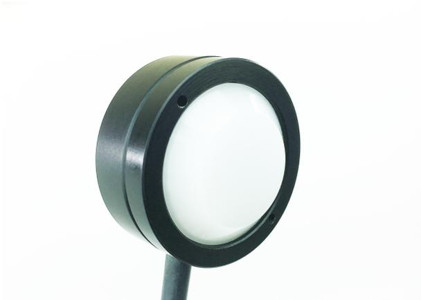
The model 268Blue is a low-profile sensor designed for applications with limited mechanical clearance. The unit is optimized for measurement in the blue portion of the spectrum, centered at 450 nm via an integrated filter, and provides Irradiance measurements in W/cm<sup>2</sup> or mW/cm<sup>2</sup>.
