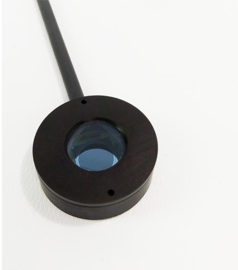
The model 268R is a low-profile sensor designed for applications with limited mechanical clearance. An integral flat filter / diffuser provides flat response from the blue to the near infrared, with measurement units of Watts or mW.
