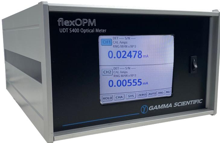
The S400 Series Optical Meters are ideal for photometric, radiometric, laser power, and fiber optic measurements. Models incorporating up to 4 individually calibrated sensor heads are available. This system features a microprocessor controlled architecture with USB, RS-232, RS-485 and IEEE-488.2 interfaces.
