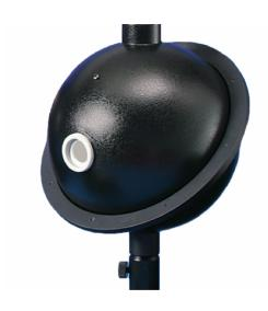
The model S2525-L Integrating Sphere has a diameter of 150 mm and a typical attenuation of 600:1. It includes an input aperture disk with a standard 5mm port and a blank adaptor which can be drilled for other aperture sizes.
