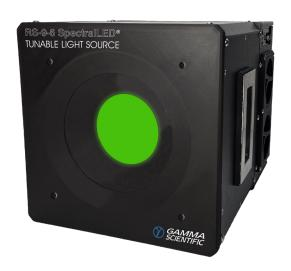
The SpectralLED® Wide Field of View (FOV) is ideally suited for applications requiring a field of view up to 180°. The unique optical design delivers equal radiance over the entire field, which is critical for users desiring flat fielding fisheye or ultra-wide FOV lens designs. With better than 95% uniformity across the 75mm output, the performance is unmatched in the industry.
